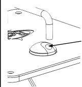
Choose one of the gromets provided the fits tightly around the cable or cables that you will be running through the gland.
