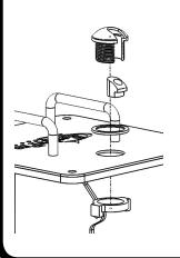
Place the cable through the black nut first, then through the cover and the seal. The top half of the gland is pushed down over the gromet and the nut is then done up finger tight on the rear.
