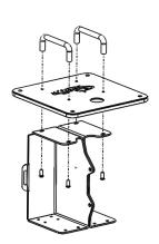
Place Loctite 246 or equivalent on the 4 M4 x 0.7 x 12 cap screws provided and screw them finger tight into the handles through the battery cradle and cover as shown.
