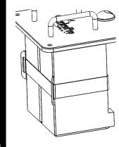
Finally install your bateries into the two cradles. (DO NOT TOUCH THE EXPOSED TERMINALS ONTO THE ALUMINIUM MOUNTS). and then wrap the velcro around the back of the mount and batteries.
