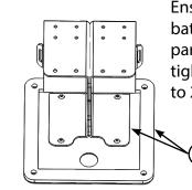
Ensure the edges of the battery cradle is running parallel with cover and tighten the 4 cap screws to 2.9 N\*m
