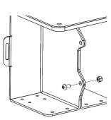
Install the M5 x 0.8 x 10 cap screw and nylock nut provided and torque to 5 N\*m.
